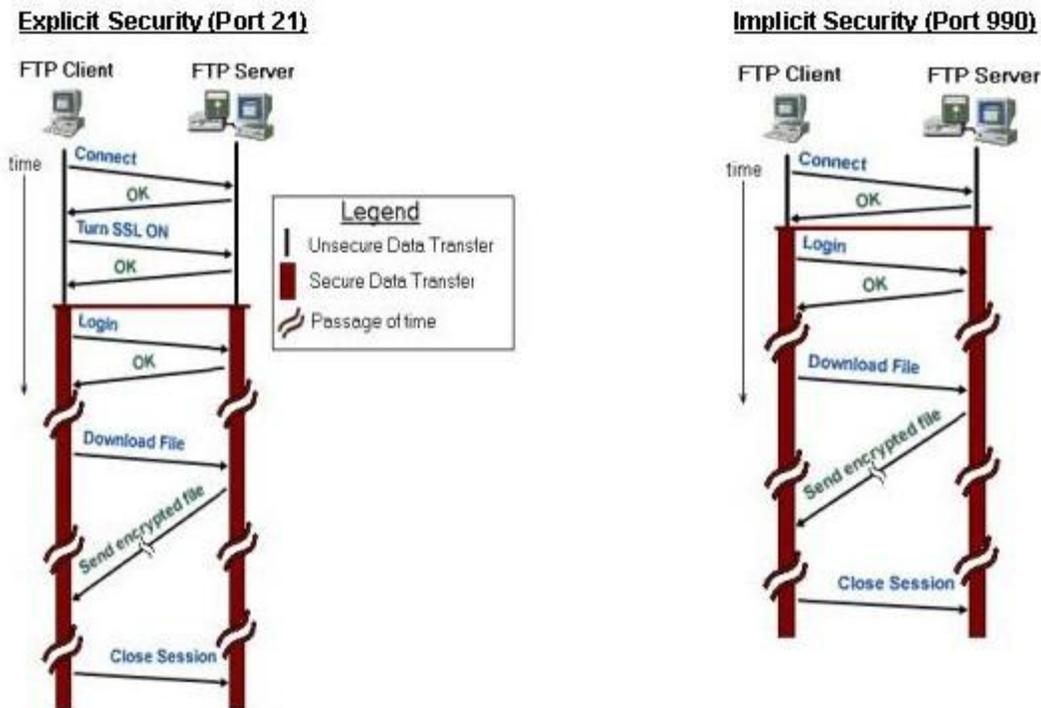
When using FTP over SSL, the control connection is encrypted and therefore unreadable for entities other than the FTP client and the FTP server. As a consequence, NAT/PAT devices and firewalls can no longer monitor the negotiation of the data connection.
